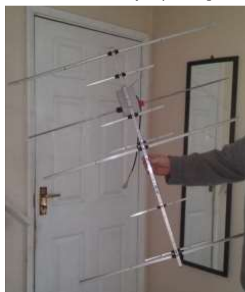
Mk2 Version of my design this one breaks down for ease of transport in the field.
