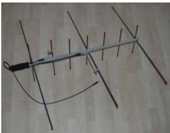
The commercially made 'Arrow Antenna' with built in diplexer. Nicely made, but still heavy!
